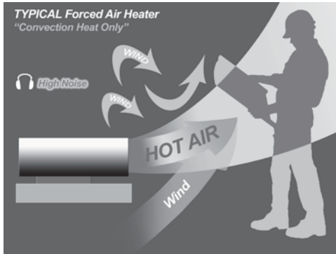
Typical Forced Air Heater
